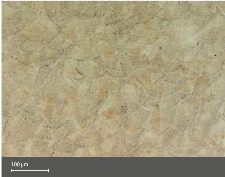
As manufactured microstructure. Etchant: Kalling's II
