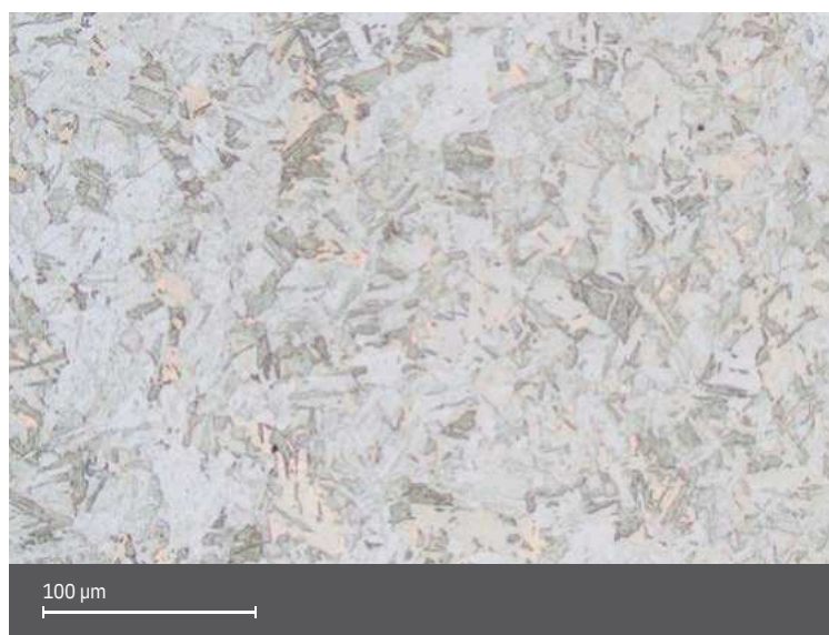
Heat treated microstructure. Etching; ASTM E407-94
