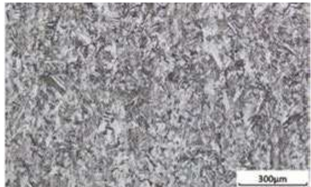
Atmospheric furnace (Atmospheric HT) was used to heat treat etched part. Etchant: Marble's reagent. 10 X magnification
